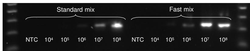
**Figure 3:** 231bp fragment of pBR322 amplified using the standard PCR mix and fast PCR mix: **Fast program:** initial denaturation 95°C for 10 min; 35 cycles of 96°C for 3s; 58°C for 3s; 68°C for 5s; final extension of 72°C for 10s. The numbers shown are the copies of template added to each 20µl reaction. NTC is a no template control.
